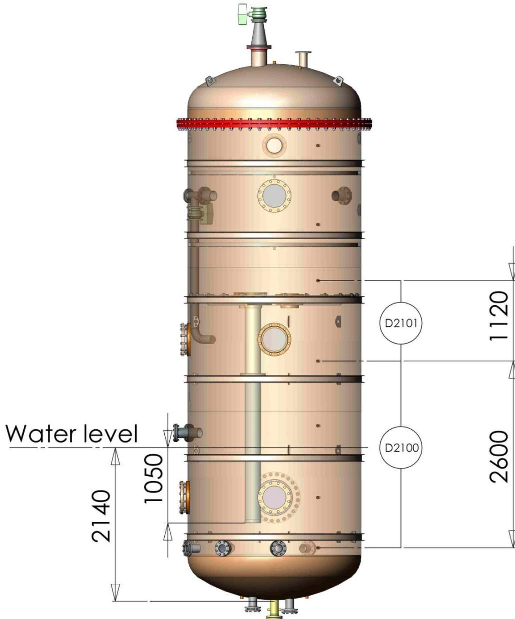
*Pressure difference measurements. Nominal water level is 2.14 m.*
