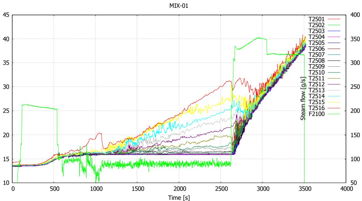
Figure 12. Temperatures in wet well water and steam flow in MIX-01.
