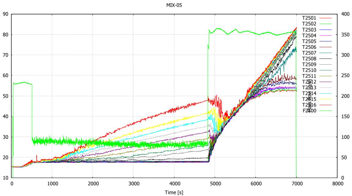
Figure 7. Temperatures in wet well water (T2501–T2516) and steam flow rate (F2100) in MIX-05.
