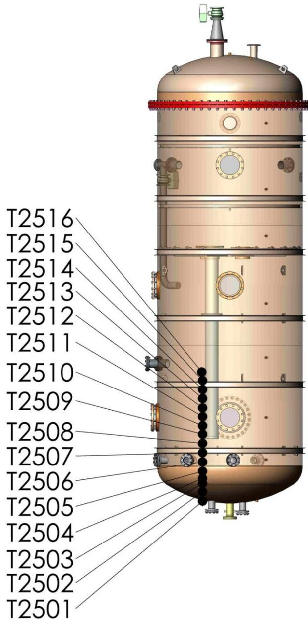
*Temperature measurements in the wet well pool for the detection of thermal stratification.*
