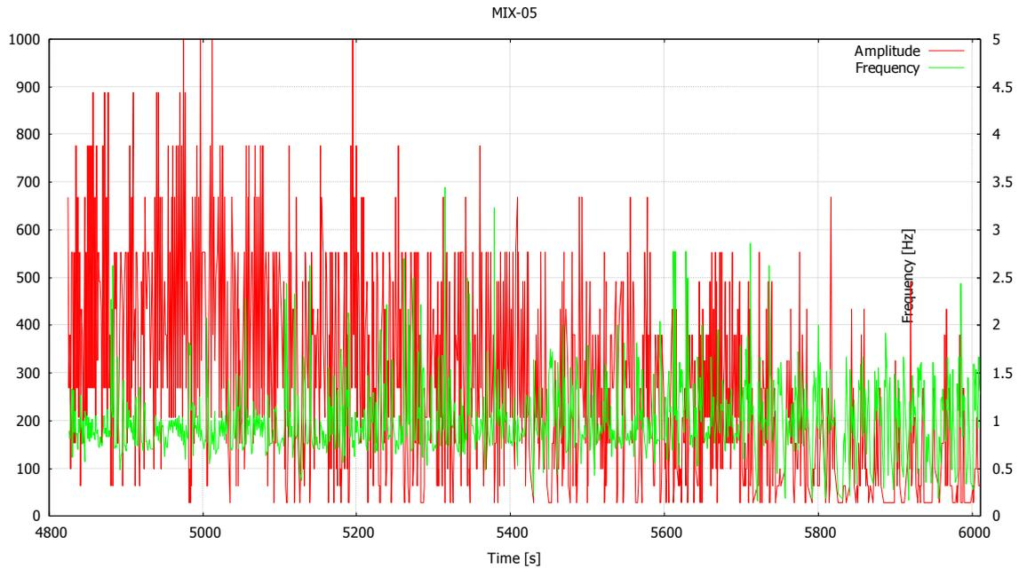
Figure 15. Amplitude and frequency of the oscillation of steam/water-interface inside the blowdown pipe in MIX-05 between 4 825...6 010 s.
