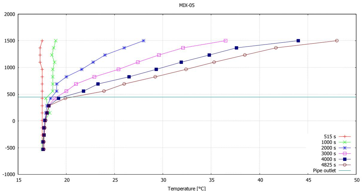
Figure 8. Development of vertical temperature profile of pool water in MIX-05.
