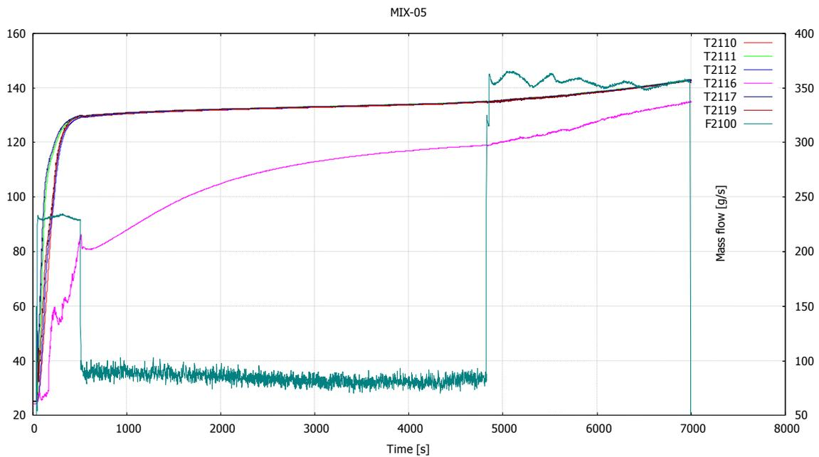
Figure 6. Dry well structural temperatures (T2110–T2119) and steam flow (F2100) in MIX-05.
