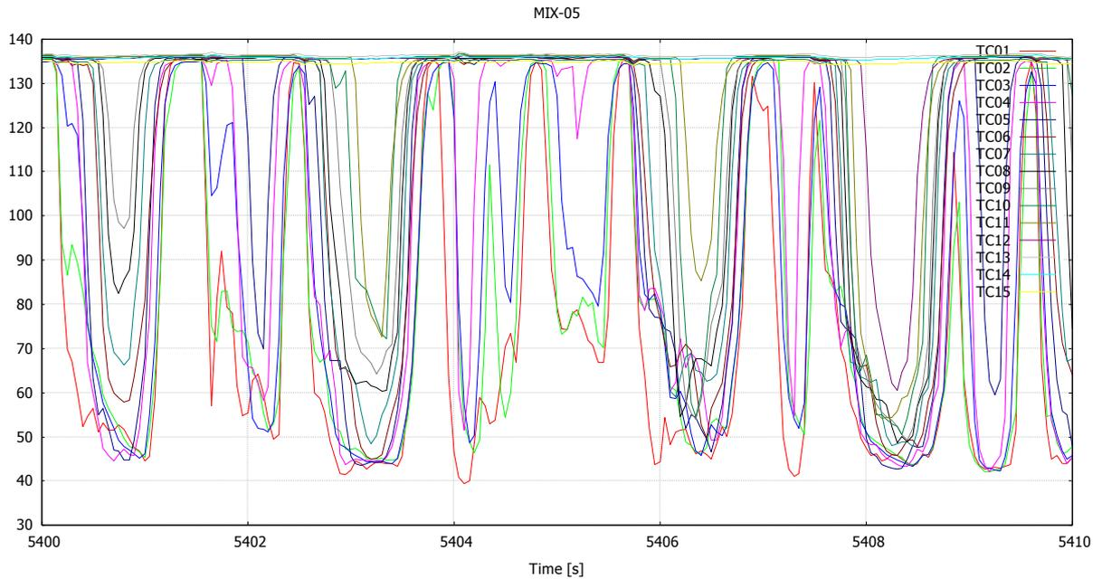
Figure 18. Temperatures inside the blowdown pipe in MIX-05 between 5 400...5 410 s.
