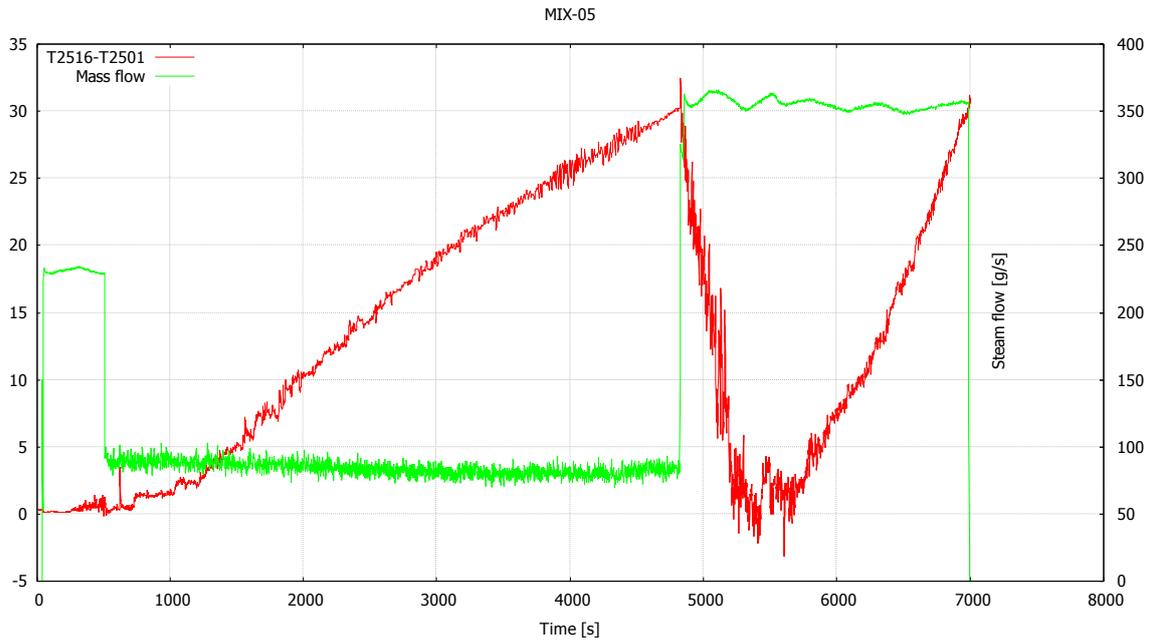
Figure 9. Temperature difference between the bottom and surface of the condensation pool (T2516–T2501) and steam flow (F2100) in MIX-05.
