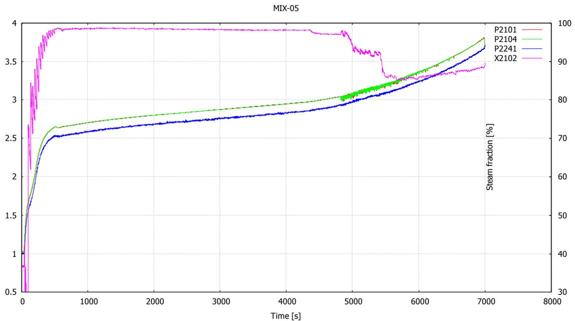
Figure 4. Pressure build-up in the test vessel in MIX-05.
