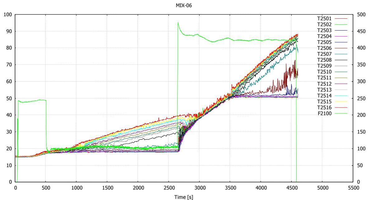
Figure 14. Temperatures in wet well water and steam flow in MIX-06.
