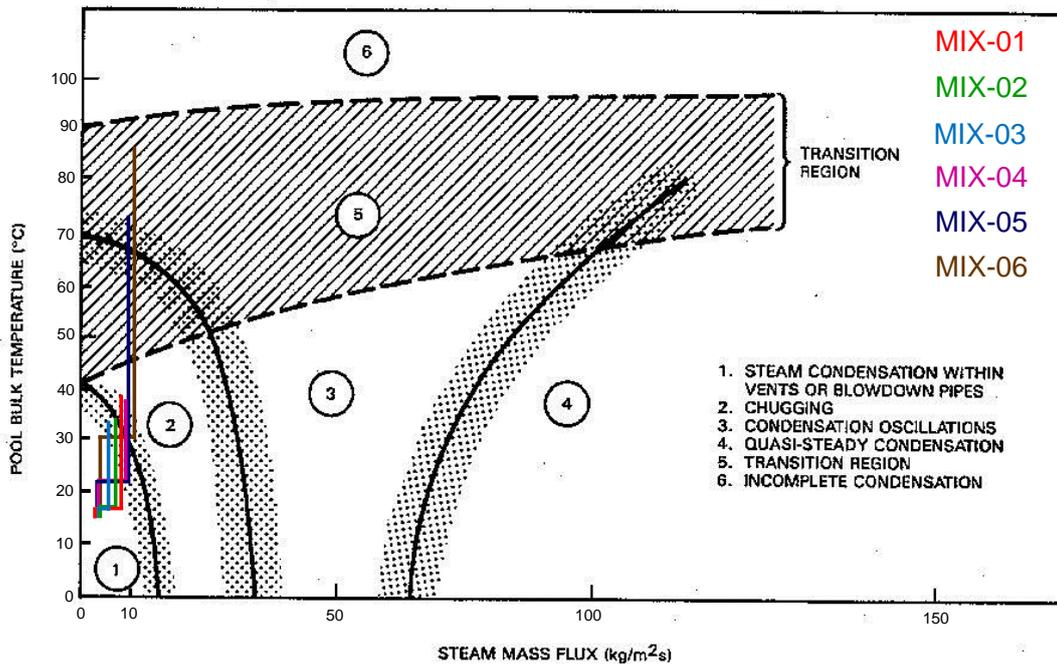
Figure 3. Condensation mode map for pure steam discharge [17].
