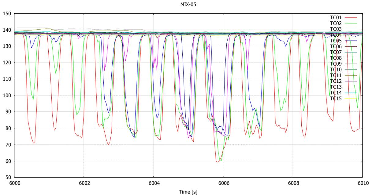
Figure 19. Temperatures inside the blowdown pipe in MIX-05 between 6 000...6 010 s.
