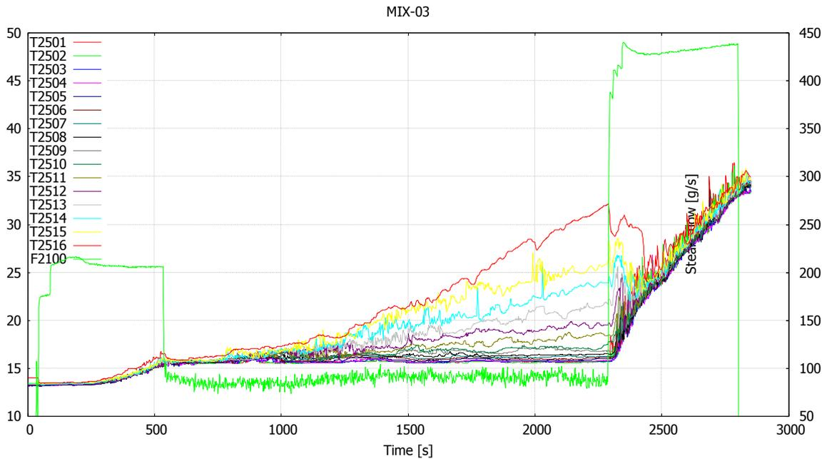
Figure 13. Temperatures in wet well water and steam flow in MIX-03.
