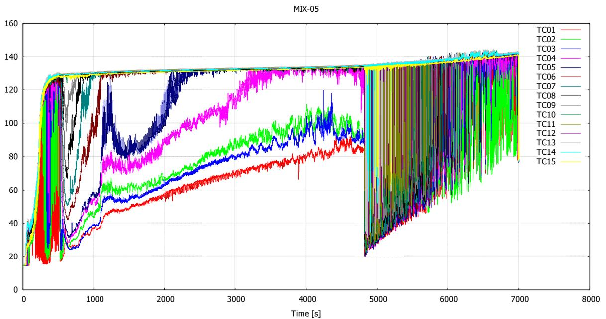
Figure 16. Temperatures inside the blowdown pipe in MIX-05.
