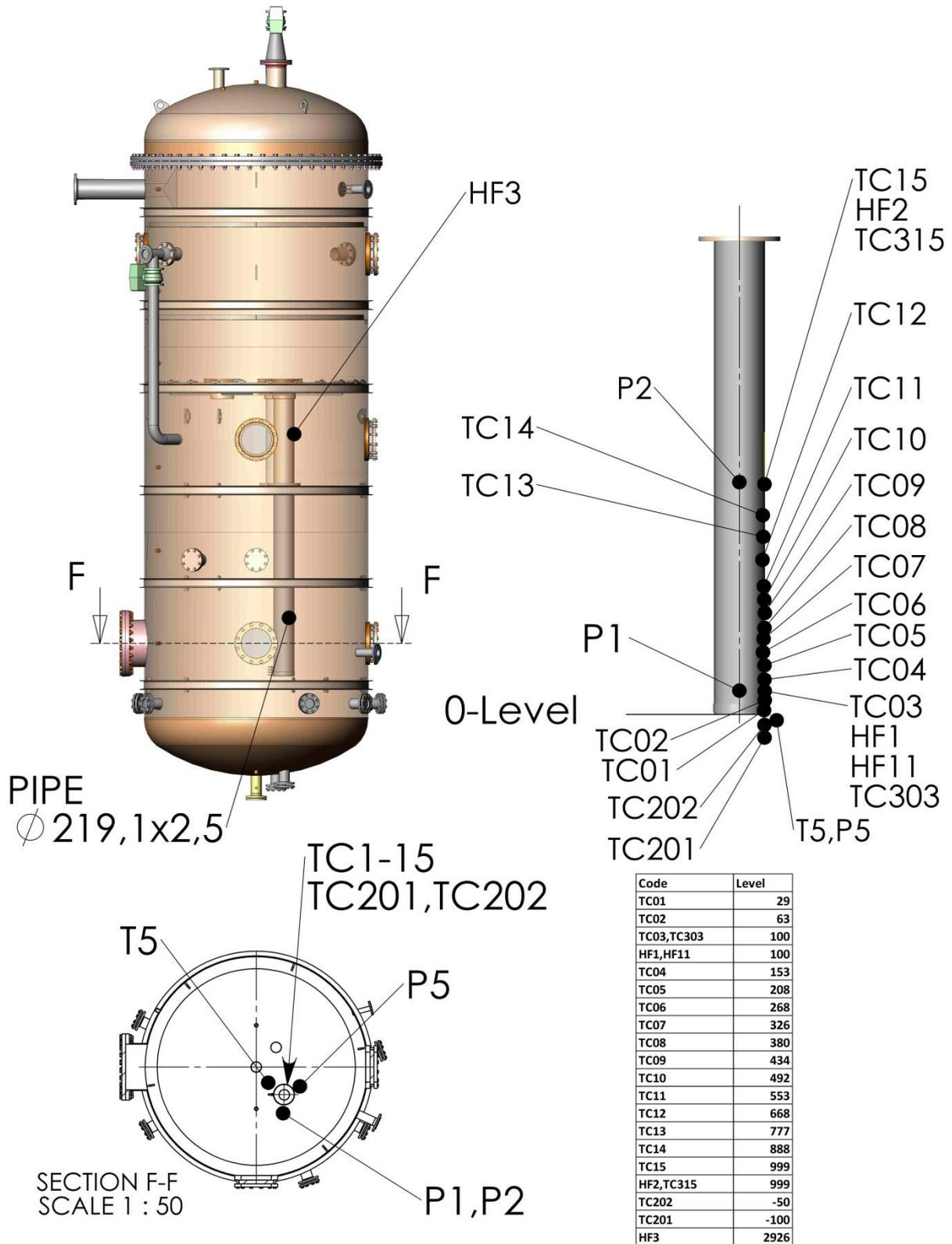
*Blowdown pipe measurements in the MIX test series.*
