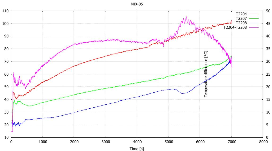
Figure 5. Thermal stratification in the wet well gas space in MIX-05.
