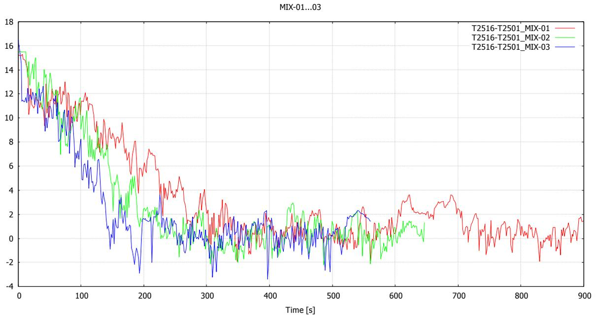
Figure 11. Temperature difference between the bottom and surface of the condensation pool ( $T_{2516}-T_{2501}$ ) in MIX-01...03. 0 s is the moment when the steam flow rate was increased to mix the pool water inventory.
