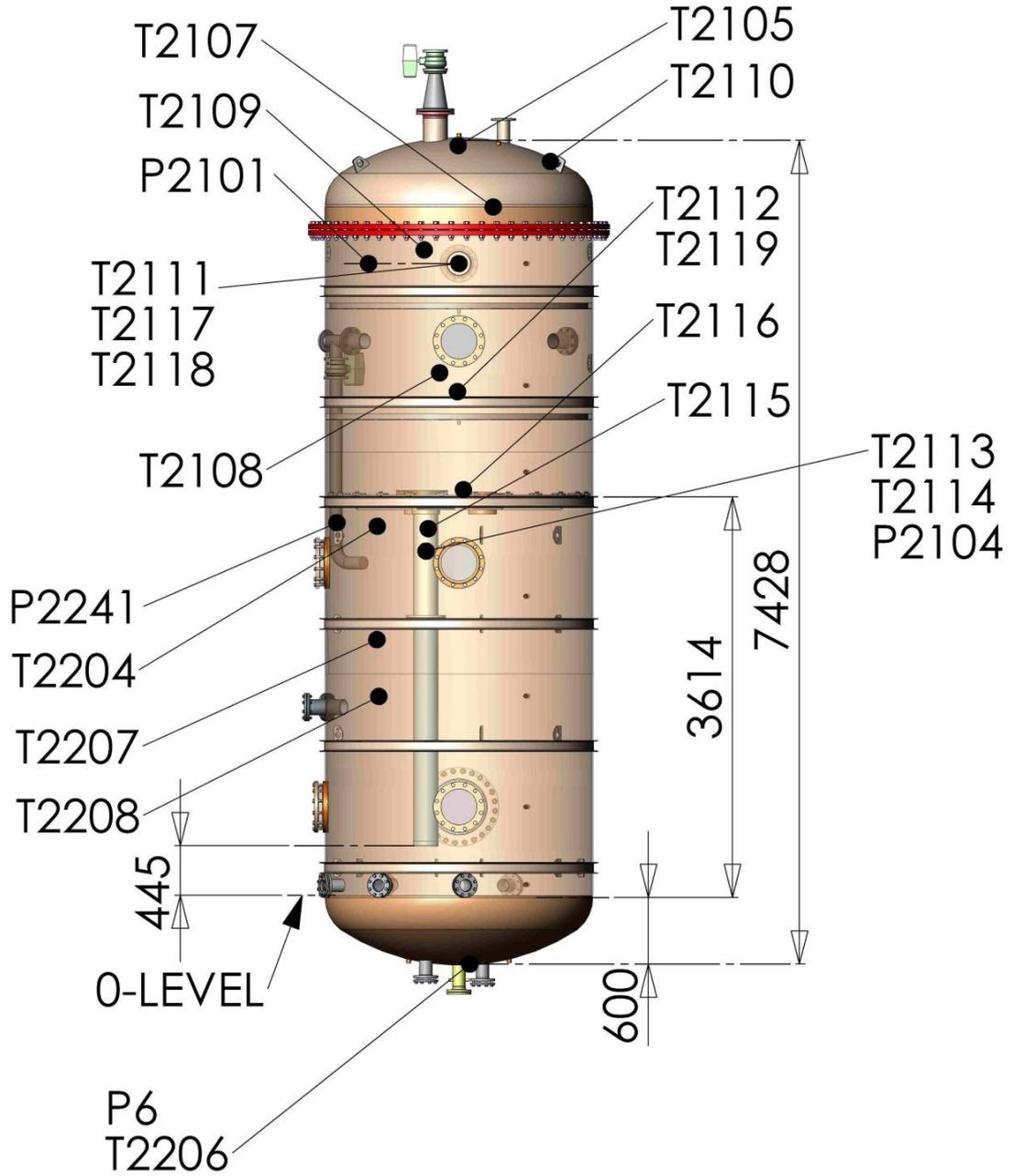
*Test vessel measurements.*
