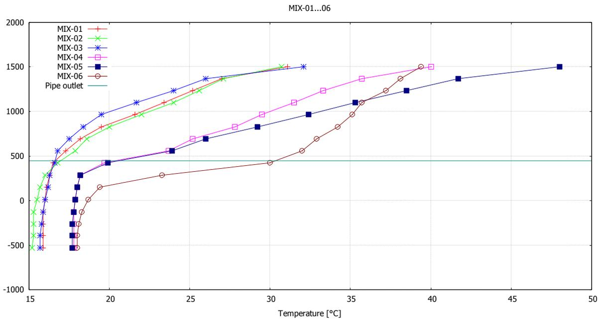
Figure 10. Vertical temperature profile of pool water in the end of the stratification period in MIX-01 ...06 tests.
