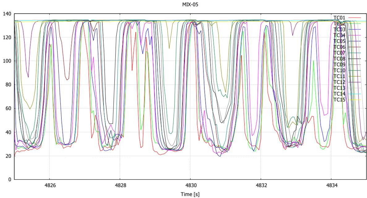
Figure 17. Temperatures inside the blowdown pipe in MIX-05 between 4 825...4 835 s.
