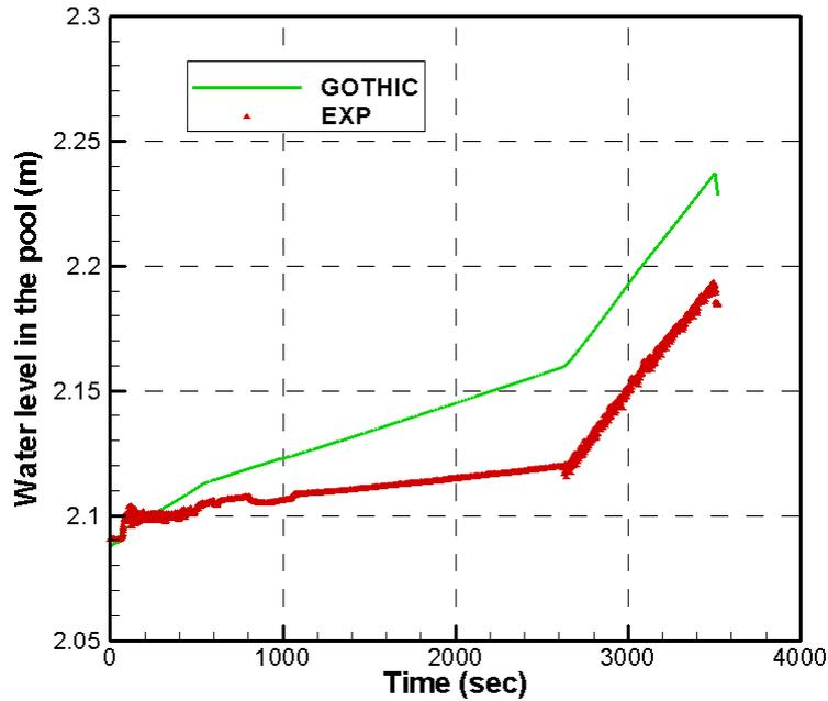
Figure 64: comparison of pool water level in GOTHIC and experiment
