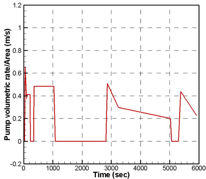
Figure 40: Pump speed used in 2D simulation with EMS model
