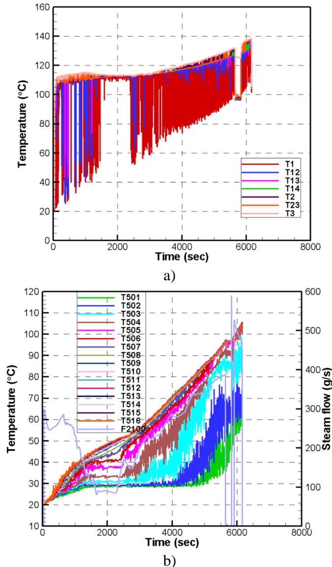
Figure 16: The data in test STR-09, a) temperature in the pipe; b) temperature history and steam flow
