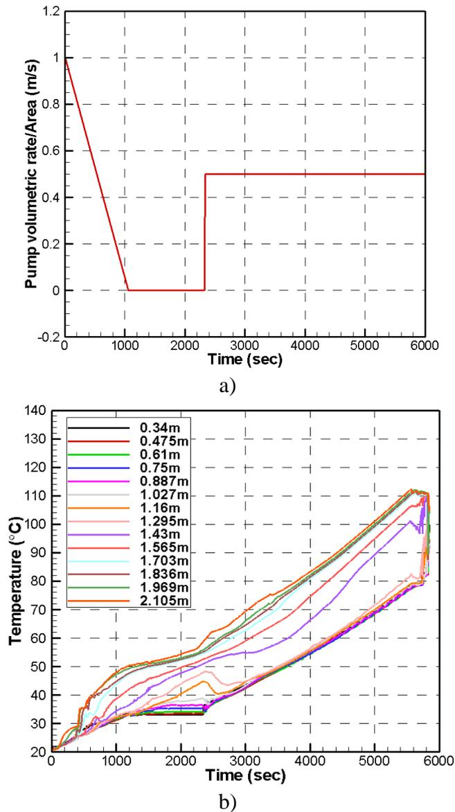
Figure 33: a) pump speed used in case 1 and b) the simulation results
