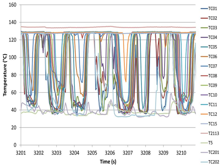
Figure 69: Temperature measured inside the blowdown pipe between 3201 s and 3211 s.
