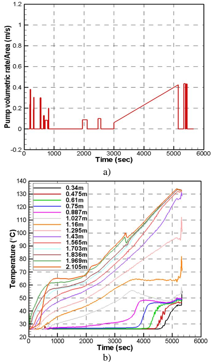
Figure 35: a) pump speed used in case 3 and b) the simulation results
