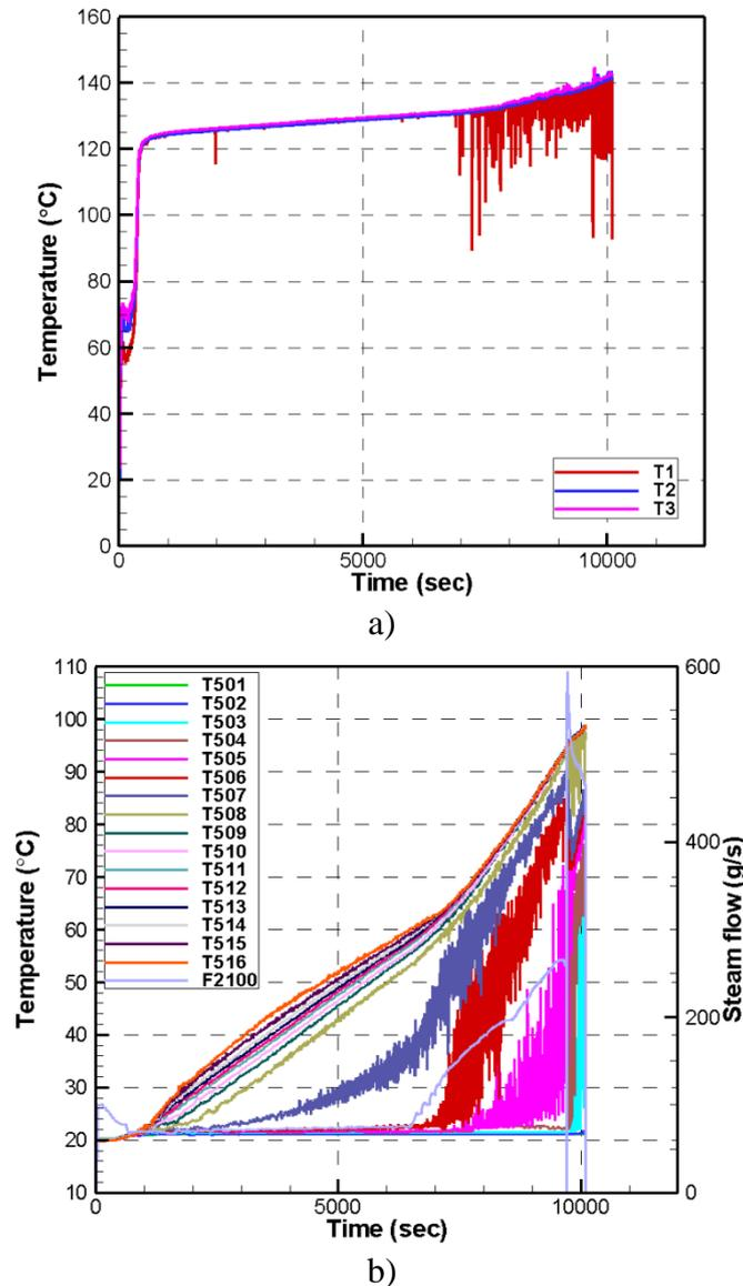
Figure 15: The data in test STR-08, a) temperature in the pipe; b) temperature history and steam flow
