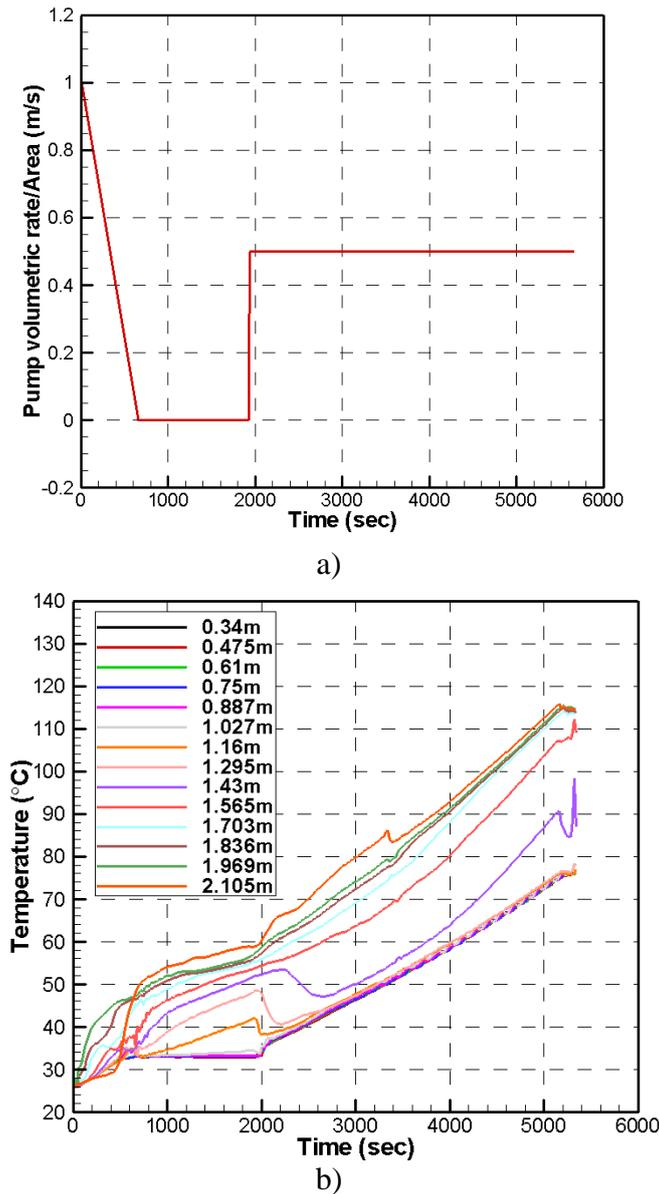
Figure 34: a) pump speed used in case 2 and b) the simulation results
