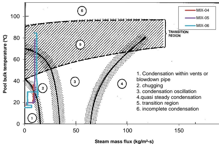
Figure 62: Condensation regimes of MIX-B tests (MIX-04, MIX-05, MIX-06)
