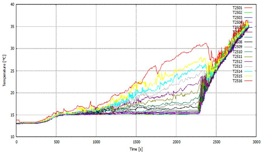
Figure 53: Pool temperature in MIX-02 (Mixing time scale: ~250 s)
