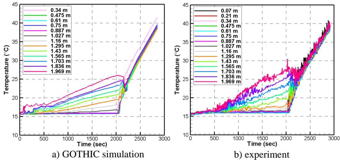
Figure 71: MIX-01 Pool temperature. a) predicted in the post-test simulation; b) measured data provided by LUT.
