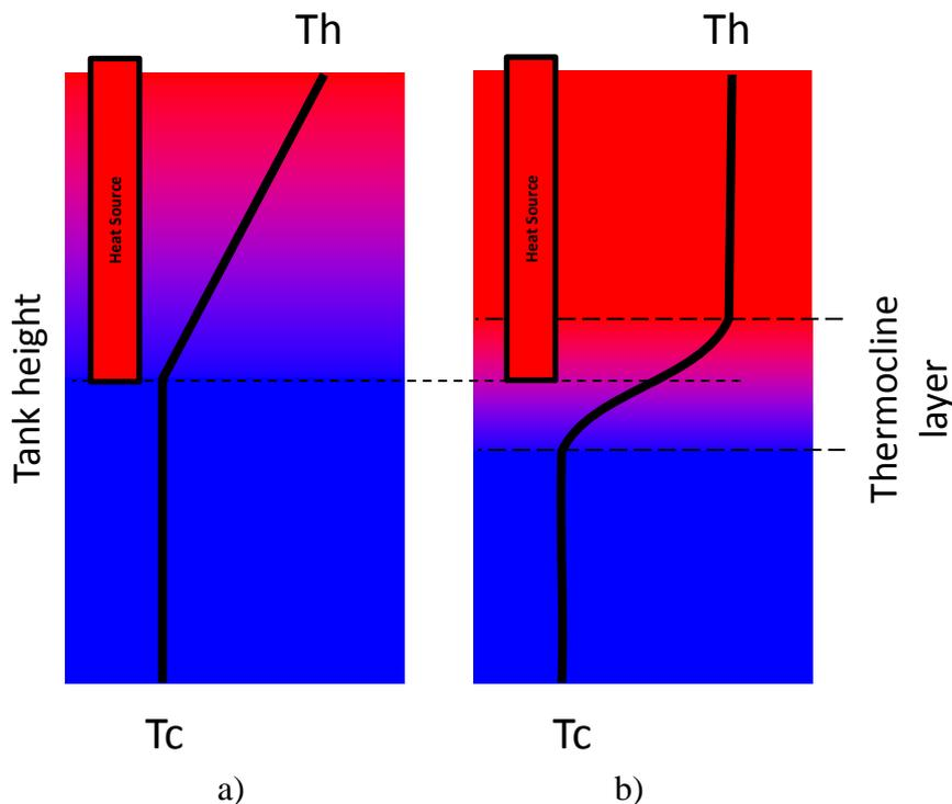
Figure 1: Typical configurations of thermal stratification in a tank:
