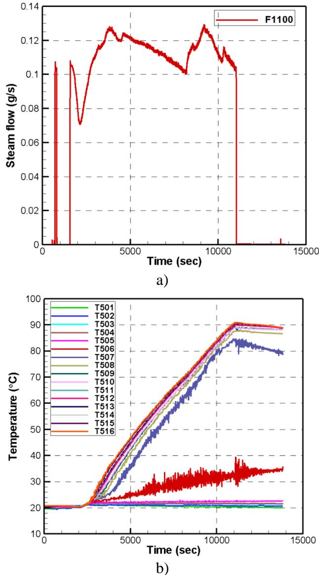
Figure 9: The data in test STR-02, a) steam mass flow rate; b) temperature history
