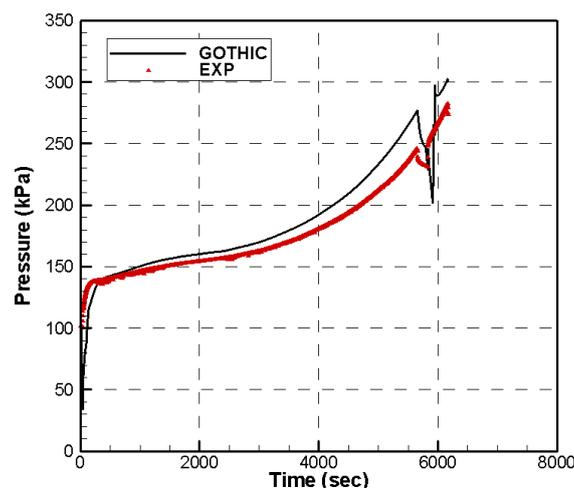
Figure 31: Comparison of calculated and measured drywell pressure.
