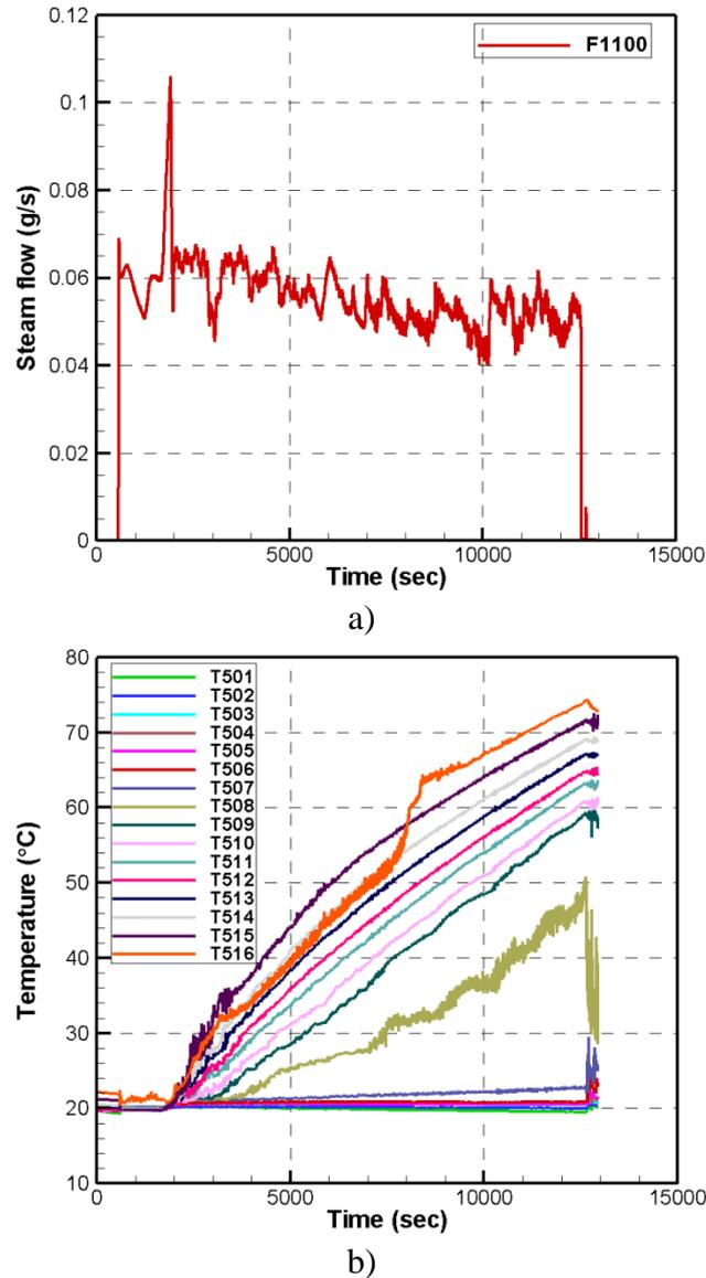
Figure 11: The data in test STR-04, a) steam mass flow rate; b) temperature history
