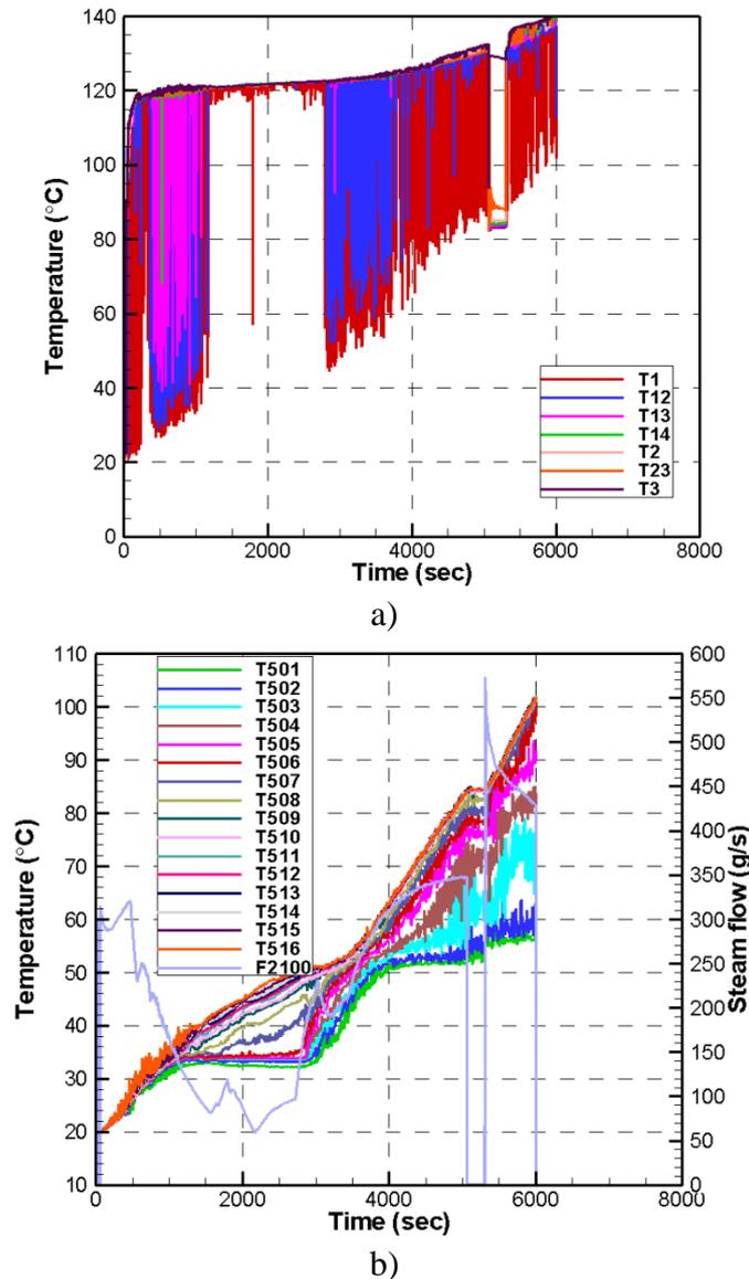
Figure 17: The data in test STR-10, a) temperature in the pipe; b) temperature history and steam flow
