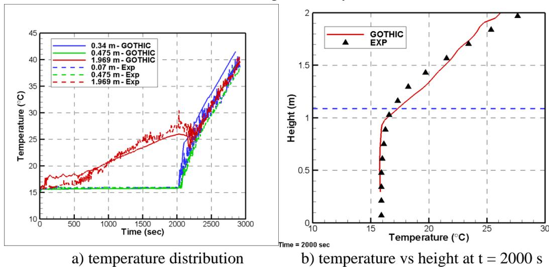
Figure 72: Comparison of predicted pool temperature in the post-test simulation with measured data provided by LUT.
