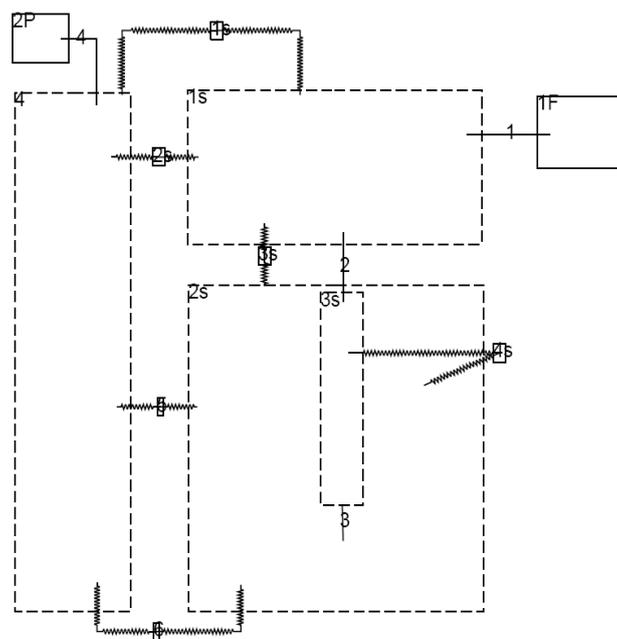
Figure 44: GOTHIC modeling scheme for pre-test simulation of the clearing phase
