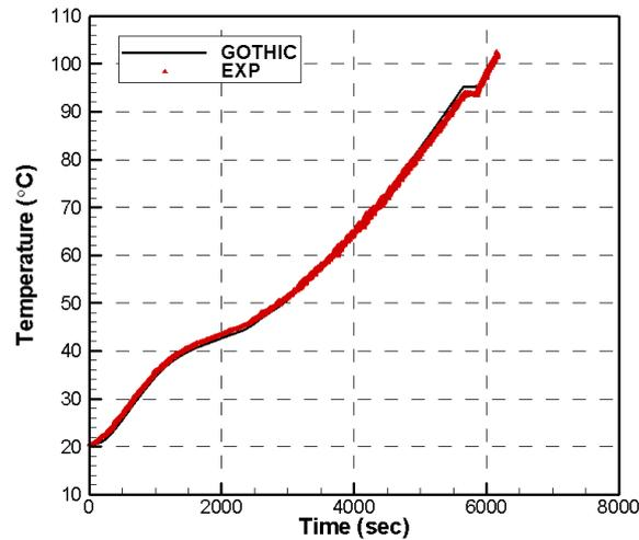
Figure 32: Comparison of calculated and measured liquid temperature in the wetwell pool.
