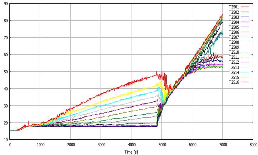
Figure 60: Pool temperature in MIX-05 (Mixing time scale: ~500 s)
