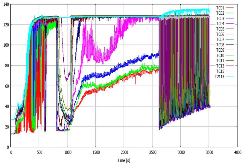
Figure 68: Temperature measured inside the blowdown pipe in MIX-01
