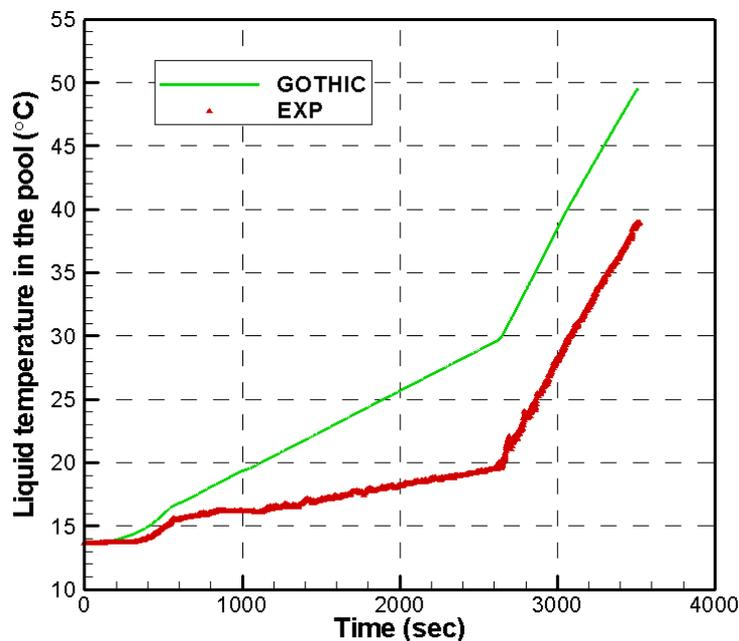
Figure 63: comparison of pool average liquid temperature in GOTHIC and experiment
