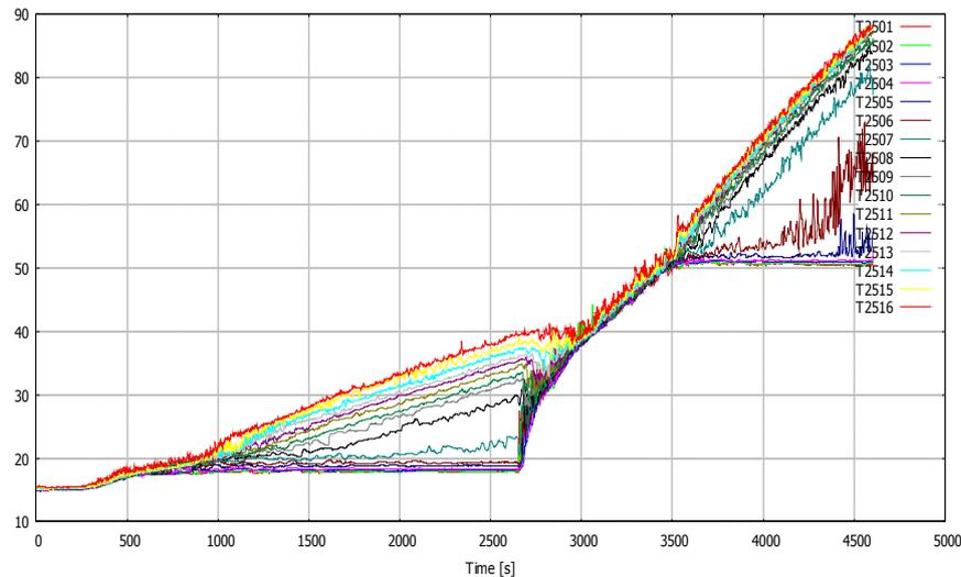
Figure 61: Pool temperature in MIX-06 (Mixing time scale: ~300 s)
