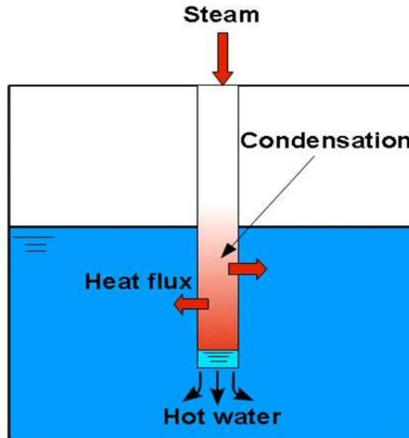
Figure 3: Schematic of Effective Heat Source (EHS) model.
