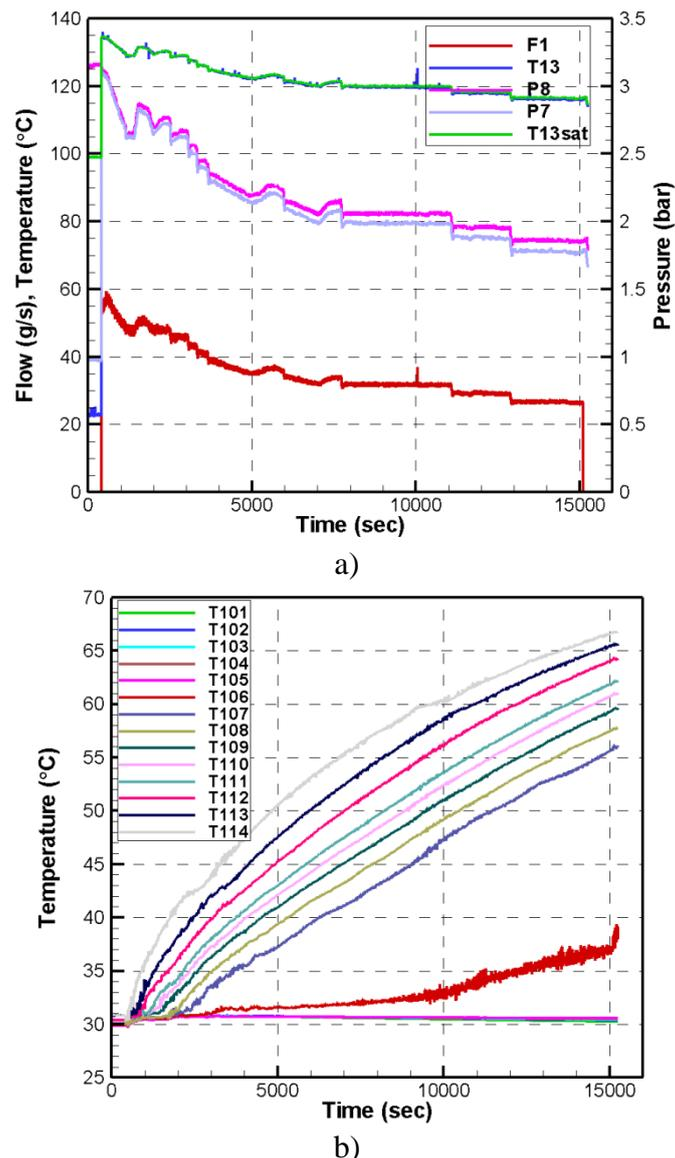
Figure 7: The measured data in STB-20, a) steam conditions; b) temperature history for heating phase with steam injection.
