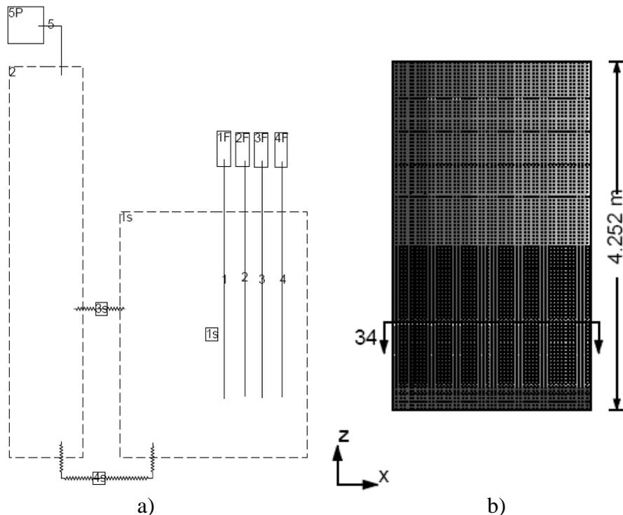
Figure 25: GOTHIC 2D modeling and grid resolution for wetwell.
