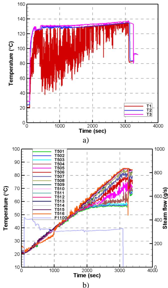
Figure 12: The data in test STR-05, a) temperature in the pipe; b) temperature history and steam flow
