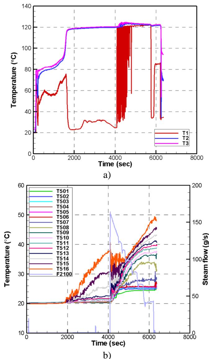
Figure 14: The data in test STR-07, a) temperature in the pipe; b) temperature history and steam flow
