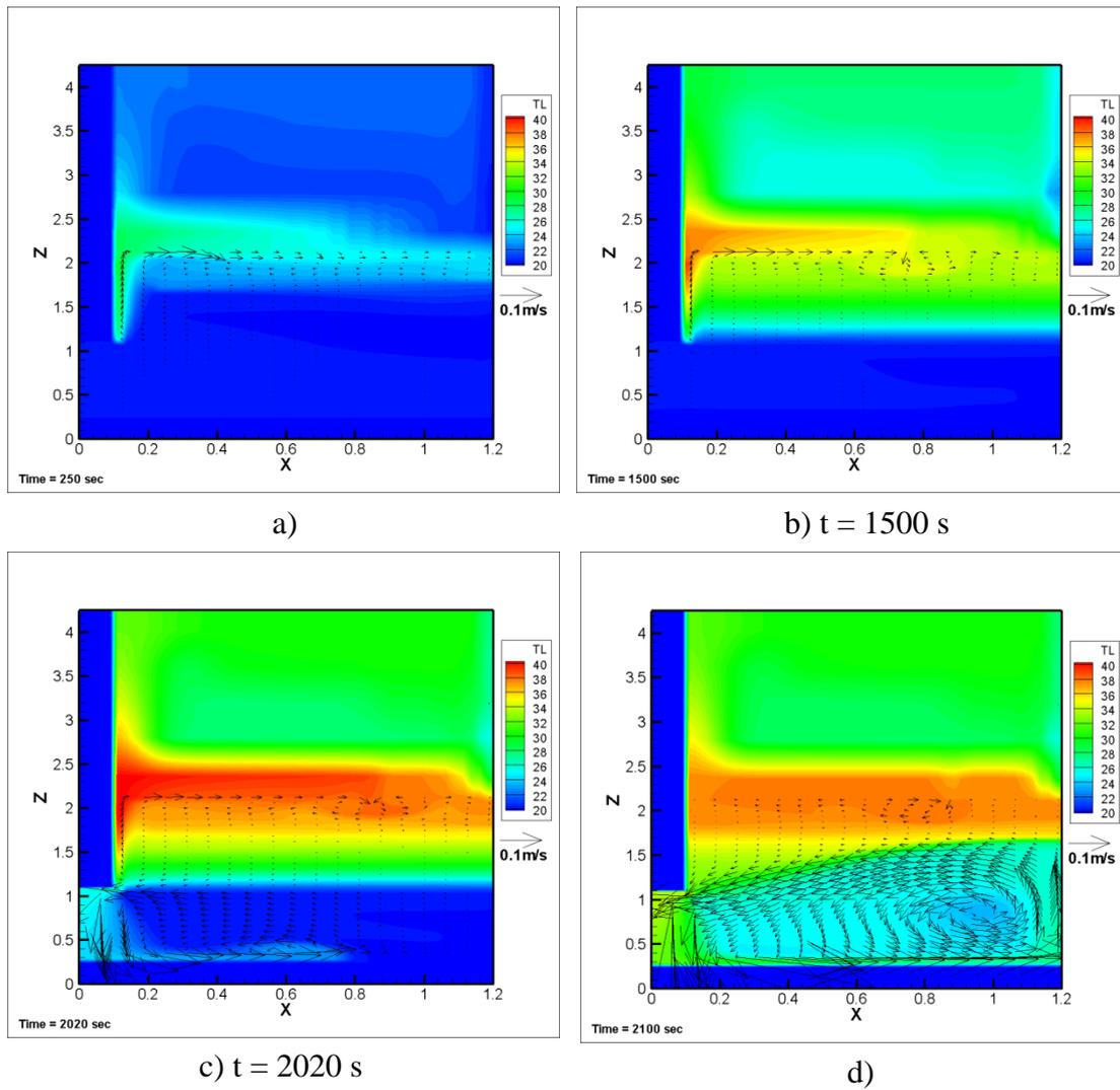
Figure 48: temperature contour and velocity vector in the tank predicted in the simulation.
