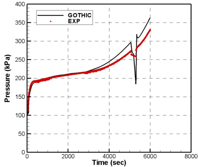
Figure 38: Comparison of predicted drywell pressure to measured pressure
