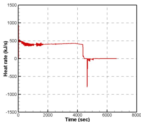
Figure 26: The heat source based on steam mass flow rate through the blowdown pipe
