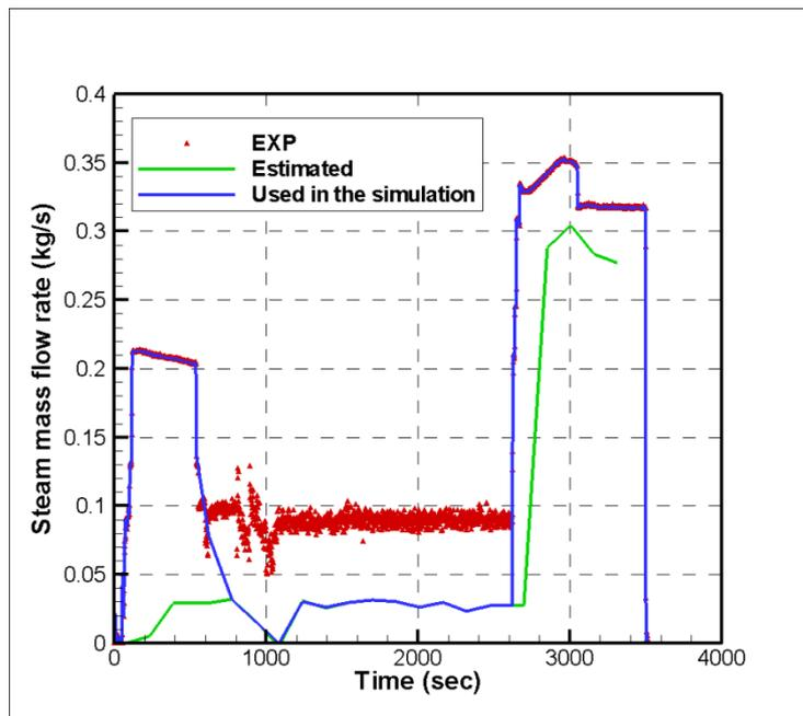
Figure 65: Comparison of steam mass flow measured in the experiment and estimation based on measured pool averaged liquid temperature.
