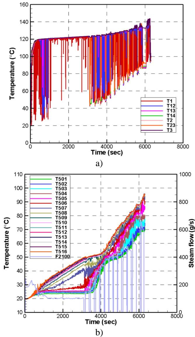
Figure 18: The data in test STR-11, a) temperature in the pipe; b) temperature history and steam flow
