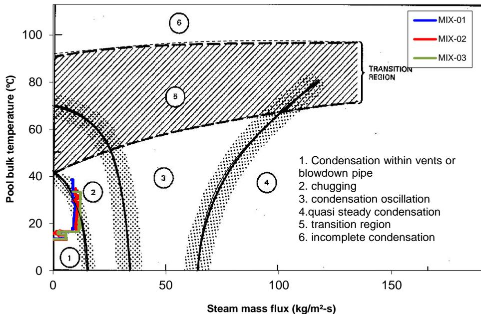
Figure 55: Condensation regimes of MIX-A tests (MIX-01, MIX-02, MIX-03)
