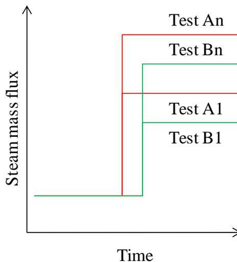
Figure 43: Schematic of the steam mass flux adjustment for the proposed tests.
