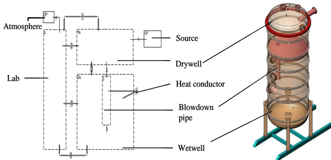
Figure 22: GOTHIC Lumped modeling for PPOOLEX facility
