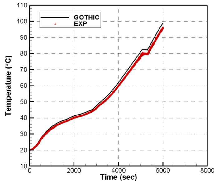
Figure 39: Comparison of predicted wetwell liquid temperature to experimental data
