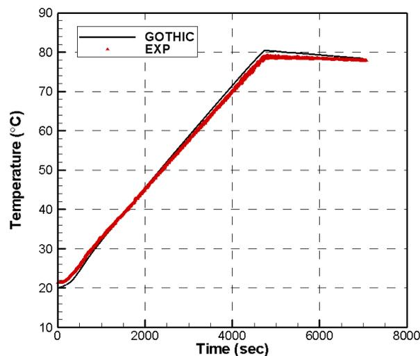
Figure 23: Comparison of predicted wetwell liquid temperature and experimental data
