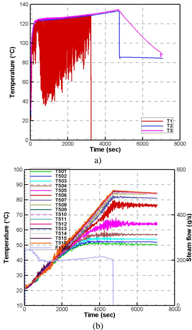
Figure 13: The data in test STR-06, a) temperature in the pipe, and b) temperature history and steam flow. The thermocouple T1 has been broken (most likely) after 3200 seconds, so no data has been recorded from this time until the end of the test.
