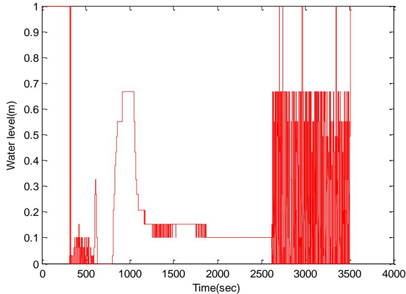
Figure 70: Water level in the blowdown pipe in MIX-01
